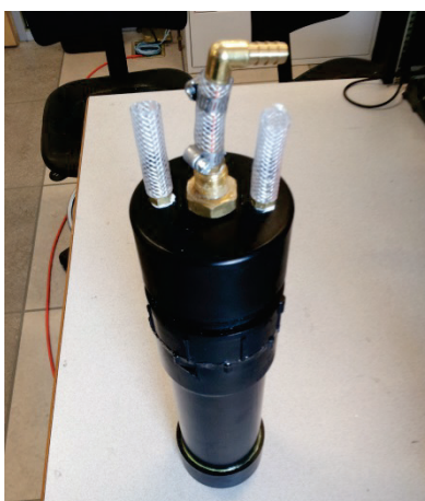
Figure 2.5. Components of custom thermo-gravimetric system: a) valve system and pressure transducer, b) filter flask with thermocouples and adsorbent sample, c) filter flask in oil bath with heater and insulation foam, d) Assembly of copper plates and cartridge heater, and e) evaporator assembly (only ABS shell visible)
