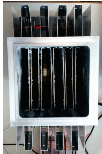
Figure 2.8. Completed adsorbent bed prototype a) isometric view with acrylic lid, and b) top view showing internal fins and gaps for vapor flow
